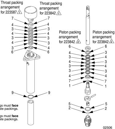
Lips of **throat** packings must **face down.** Lubricate packings.
